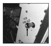
Figure 16: Water Supply Fitting
